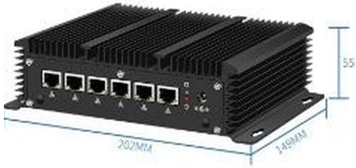
Chassis dimensions (mm)
